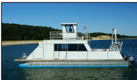
The R/V PECONIC is a U. S. Coast Guard-inspected catamaran, houseboat-style vessel for operation in protected bays and rivers.
